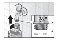
Plastic threads must only be tightened by hand. Do not remove the strainers from the water supply hose.
